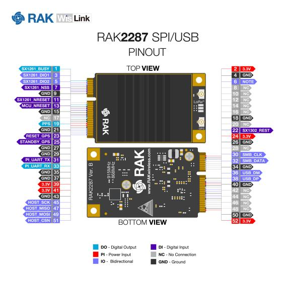
Figure 3: RAK2287 Pinout Diagram
