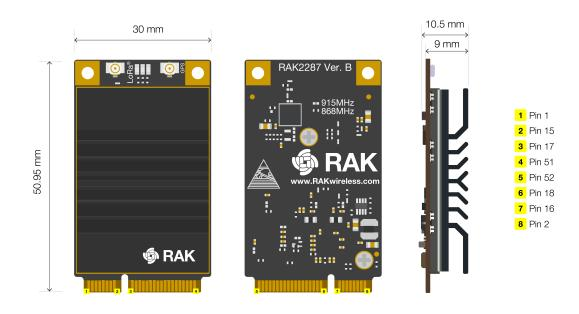
Figure 4: RAK2287 Board Dimensions
