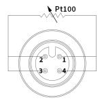
The HiTemp140-M12 is compatible with probes that have the wiring configuration as shown to the left.
